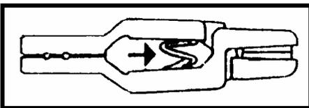
**NOTE: Make sure the spring on the OR16 clip is positioned in the heavy setting (see diagram to the left). If the spring is not in the heavy setting, move the spring toward the pads with the use of key, screwdriver, etc.**
