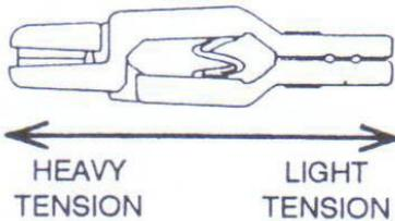
The OR31 SST Side Planer comes with one OR19 Adjustable Heavy Tension Planer Board Release. The spring in the release can be slid toward the pads to increase the tension and away from the pads to reduce the tension depending on the species or conditions to be fished. (See illustration on the left) Spring can be moved with the use of a key, screw driver, etc...
